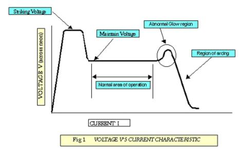
Neon lamps have a current/voltage characteristic as shown in Fig 1 above.
