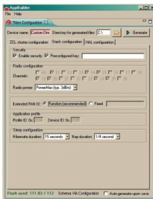
In addition to the devices and cluster selections, the developer can configure the various options associated with the ZigBee PRO stack, as allowed by the Application Profile (Home Automation Profile shown). In this example, security operation, transmitter power, PAN ID, and sleepy end device parameters are shown.
