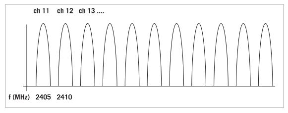
Figure 4 - The 802.15.4 2.4 GHz Spectrum
