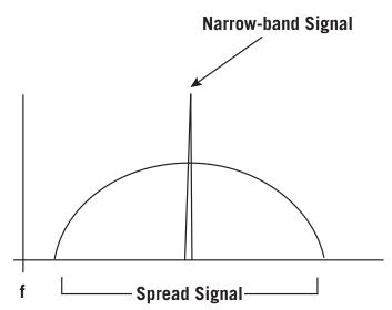
Figure 3 - Spread-Spectrum Signal
