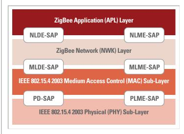
Figure 1 - The ZigBee Stack
