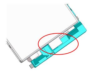
3) The guiding keys touch on the receptacle first to guide the plug correctly.
