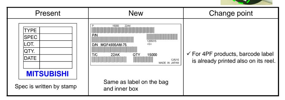
These change is only for labeling. The device performance and assembly in customer's line is not affected.
