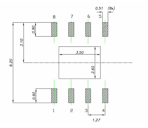
**Comment:** In spite of small difference on some dimensions, the new package is compatible with the in production one. Both package types are JEDEC compliant and can be indiscriminately used with above recommended footprint.
