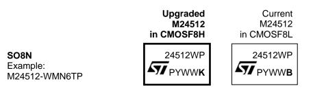
For **TSSOP8**, the difference is visible inside the product name: **upgraded version** in **CMOSF8H** is ending by "**K**", the current version was ending by "P".
