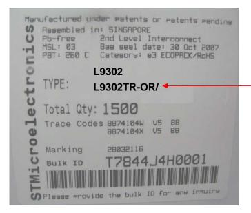
The two characters "OR" will be introduced among the last characters of the Finished Good code to identify a carrier tape with the new orientation.
