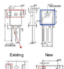
New Supplier has different dimension and shape on body notch area compared to Littelfuse Original POD
