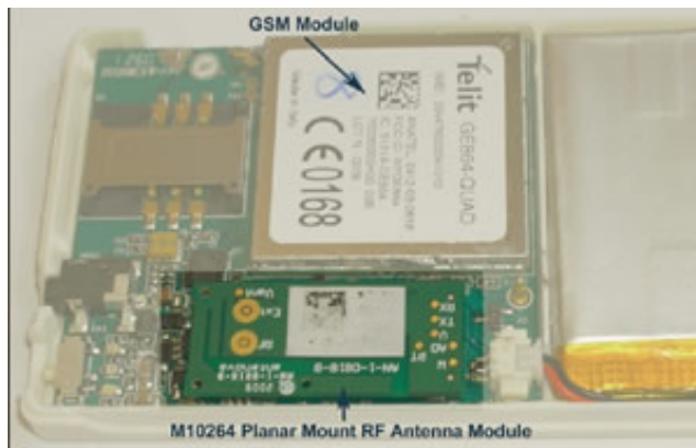
Figure 1: An 80x50x6.9mm tracker device with GPS RF antenna module (at the bottom of the picture).
