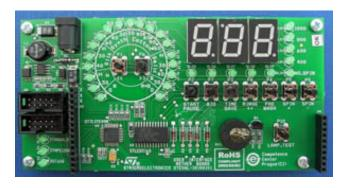
The STEVAL-IHI001V1 is a demonstration board designed to simulate the user interface of a modern white goods, such as a washing machine.
