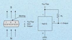
Unipolar Hall effect switches will switch on with a south magnetic field of sufficient strength. The output will switch off if the magnetic field is removed.
