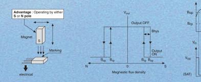
$B_{op}$ : Magnetic operate point. A positive magnetic field > $B_{op}$  will switch the sensor on (output low).  $B_{rp}$  : Release point. Removal of the magnetic field  $\langle B_{rp}$  will switch the sensor off (output high).
